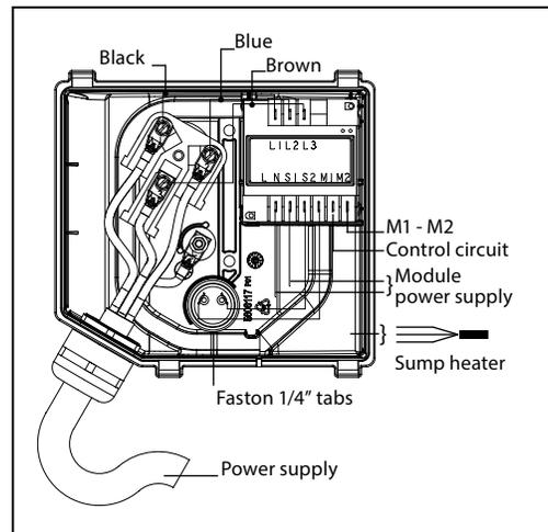
The motor protection module comes preinstalled within the terminal box. Phase sequence protection connections and thermistor connections are pre-wired. The module must be connected to a power supply of the appropriate voltage. The module terminals are 0.25" size Faston type.
