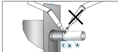
In addition, for discharge connections equipped with a non return valve integrated in discharge fitting (SY/SZ240-300) the direction of the torch has to be as described on the picture, and maximum brazing time should be less than 2 minutes to avoid NRVI damages.
