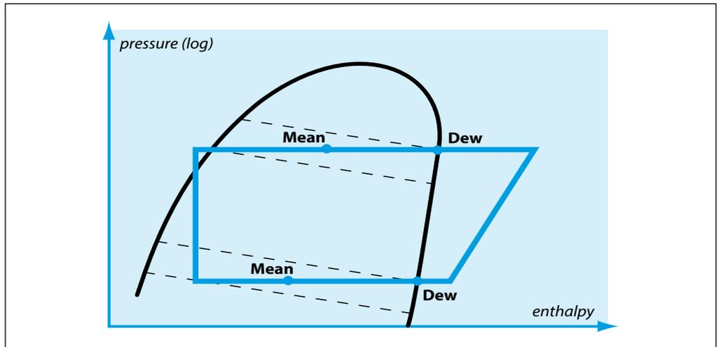
The following operating diagrams show the difference between mean and dew temperature application envelopes.
