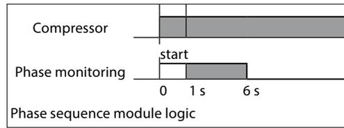
The lockout may be cancelled by resetting the power mains (disconnect L-N) for approximately 5 sec.
