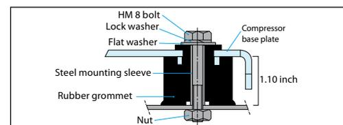
**Mounting of SM/SZ 112-124-147:** the required bolt size is HM8. This bolt must be tightened to a torque of 11 ft/lbs. The bolt and washers are supplied with the assembly kit. When a surface sump heater is used, it must be applied after grommets are mounted on compressor in order to avoid surface sump heater damage.
