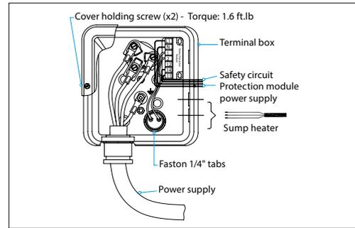
The motor protection module comes preinstalled within the terminal box and has pre-wired thermistor connections. The module must be connected to a power supply of the appropriate voltage. The module terminals are 0.25" size Faston type except for 24V DC module (screw connection).
